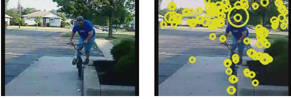
Figure 1. Camera motion can make lots of sparse feature points fall into background. Left is a frame in a bike trick video, right shows the detected feature points by STIP
